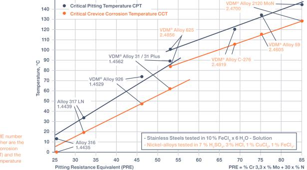
The higher the PRE number of an alloy the higher are the Critical Crevice Corrosion Temperature (CCT) and the Critical Pitting Temperature (CPT)
