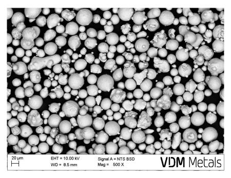
The picture shows a typical micrograph of VDM® Powder 59 as an example.
